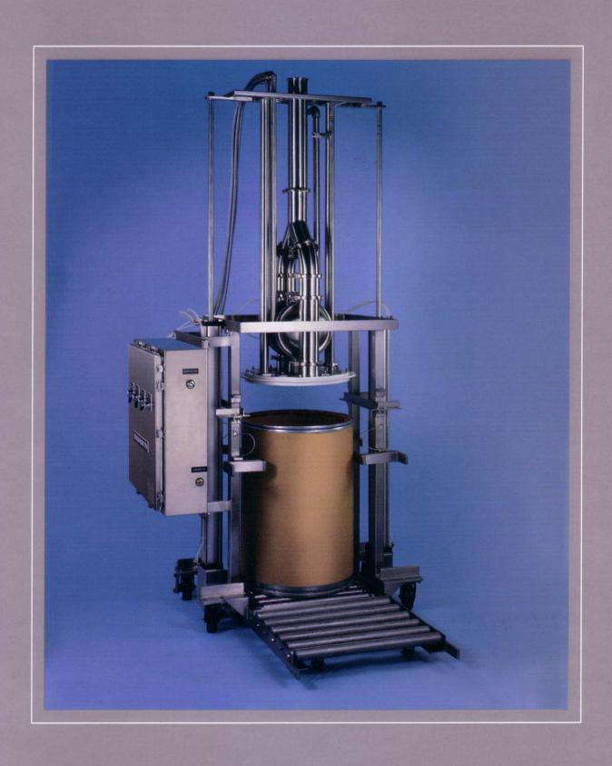
The Murzan DUS-50 is the ultimate solution for emptying the most viscous materials from 55-gallon drums or containers of any shape. When used in applications which no pump alone could handle, the system empties the containers quickly and cleanly without adding any pressure to the product or the container. The system is FDA listed and USDA approved.
